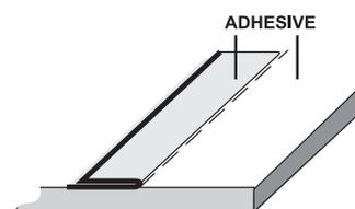
Fold back half of the sheet. Apply adhesive to both the sheet and surface.
