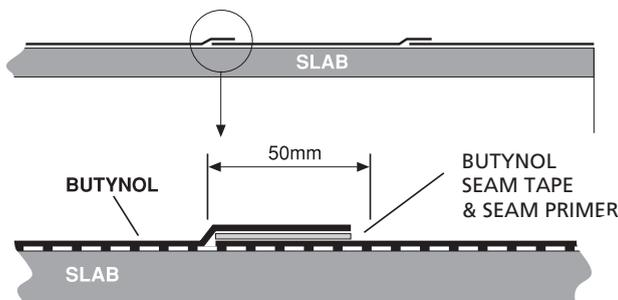
1. The top lap should be positioned 50mm over the bottom sheet and the bottom sheet should be marked to indicate where the edge of the top sheet will finish.
