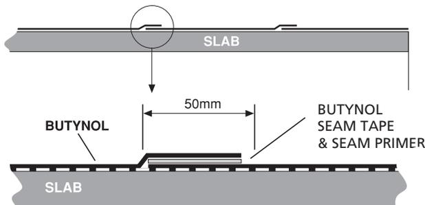
1. The top lap should be positioned 50mm over the bottom sheet and the bottom sheet should be marked to indicate where the edge of the top sheet will finish.
